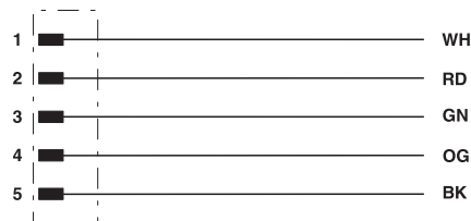
Contact assignment of 7/8" plug
