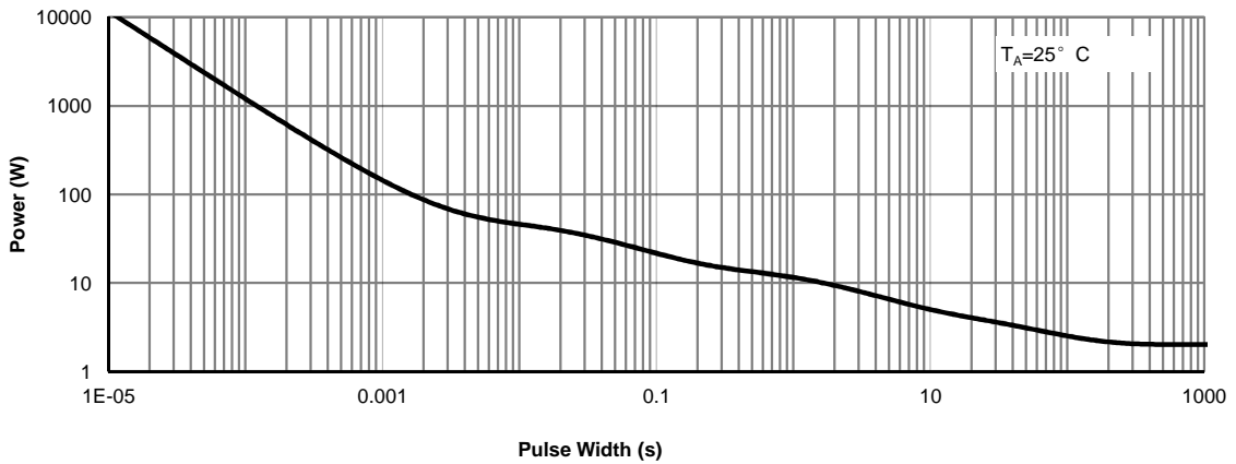
Figure 14: Single Pulse Power Rating Junction-to-Ambient (Note H)
