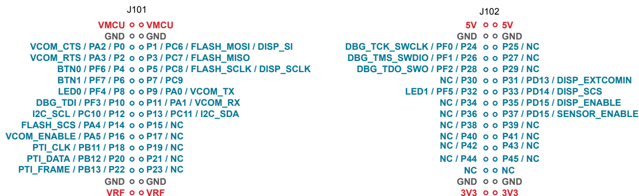
Figure 4.2. Radio Board Pin Mapping on Breakout Pads
