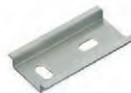
TS 35/7.5 mm according to EN 50022 (s = 1.0 mm)
