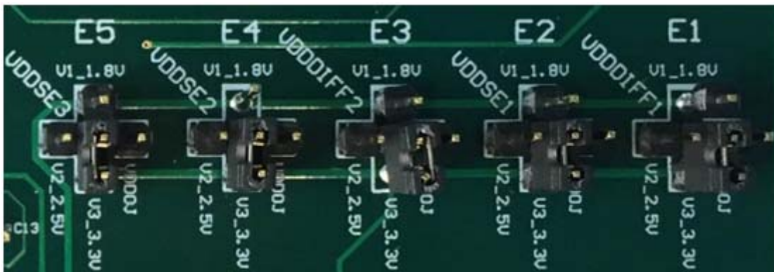
Figure 3. Jumper Configuration for On-board Voltage Regulators
