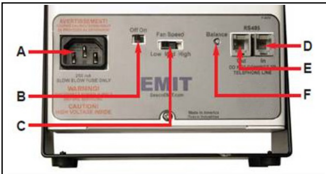
Figure 3. Bench Top Zero Volt Ionizers features and components
