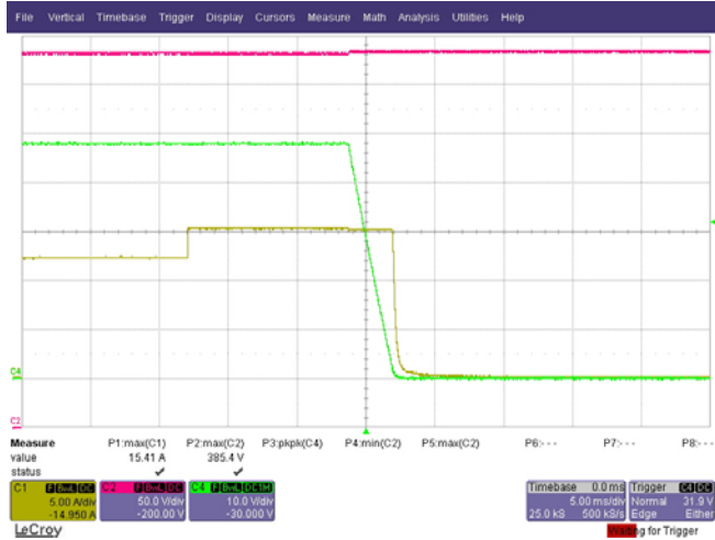
Figure 16. OCP at 385 V dc, 15 A Load (Action to Shutdown After ~10 ms) Green Trace: Output Voltage, 10 V/div, 5 ms/div Yellow Trace: Load Current, 5 A/div, 5 ms/div Red Trace: Input Voltage, 50 V/div, 5 ms/div
