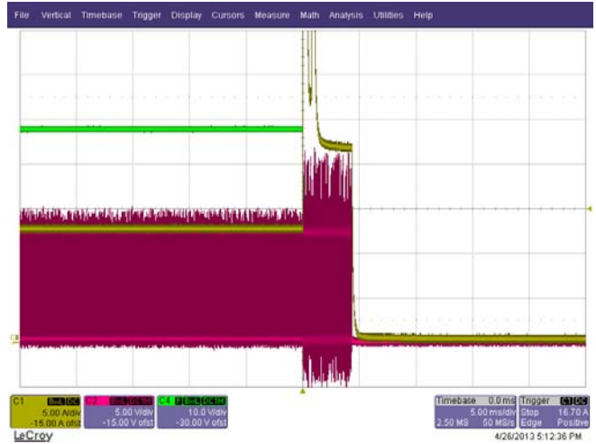
Figure 18. OCP at 385 V dc, 600 W to Output Shorted Red Trace: SR Drive, 5 V/div, 5 ms/div Green Trace: Output Voltage, 10 V/div, 200 \mu s/div Yellow Trace: Output Current, 5 A/div
