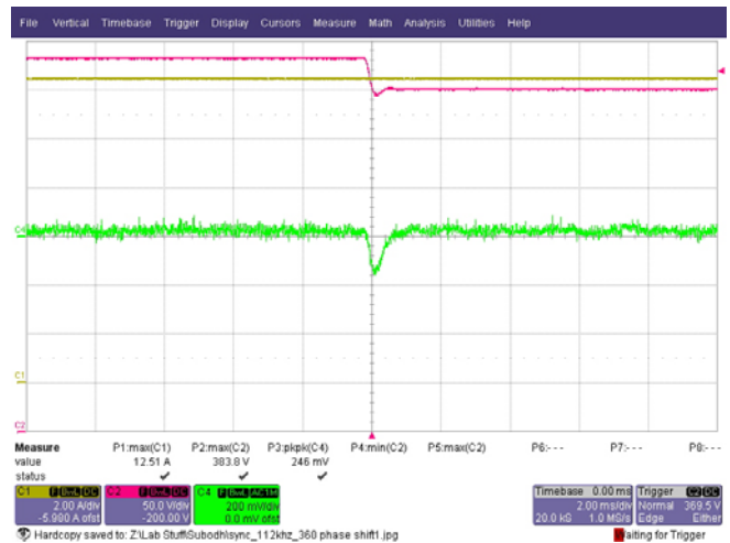
Figure 43. Line Voltage Feedforward Enabled, 600 W Load Red Trace: Input Voltage Step, 350 V dc to 385 V dc, 50 V/div Green Trace: Output Voltage (AC-Coupled), 200 mV/div
