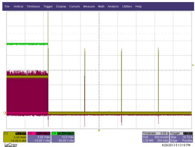
Figure 19. OCP, Hiccup Mode, 385 V dc, 600 W to Output Shorted Red Trace: SR Drive, 5 V/div, 5 ms/div Green Trace: Output Voltage, 10 V/div, 200 \mu s/div Yellow Trace: Output Current, 5 A/div
