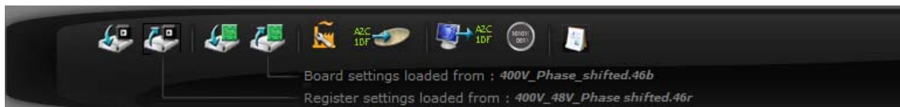
Figure 8. Different Icons on Dashboard for Loading and Saving .46r and .46b Files
