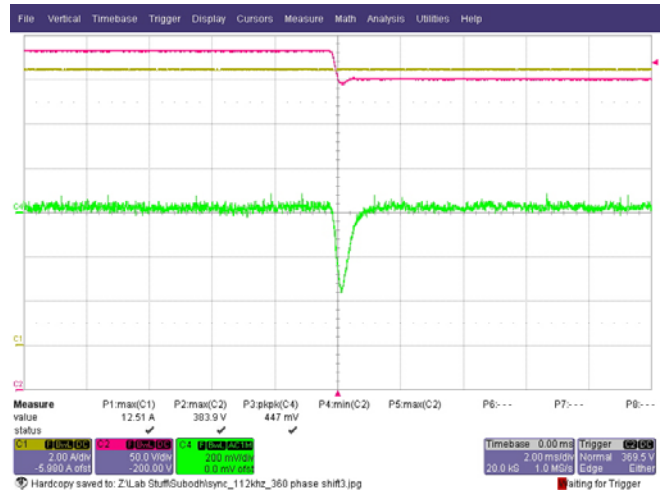
Figure 42. Line Voltage Feedforward Disabled, 600 W Load Red Trace: Input Voltage Step, 350 V dc to 385 V dc, 50 V/div Green Trace: Output Voltage (AC-Coupled), 200 mV/div
