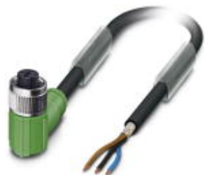
Sensor/actuator cable, 3-position, Variable cable type, shielded, free cable end, on Socket angled M12, A-coded, cable length: Free input (0.2 ... 40.0 m)
