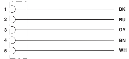
Contact assignment of 7/8" socket
