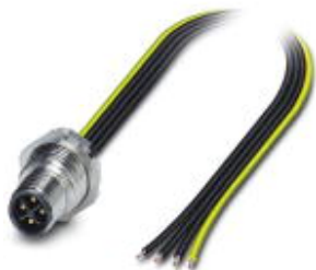
Flush-type connector, Power, 4-position, Plug, M12, S power, Rear mounting, M16 x 1.5, Individual wires, cable length: 0.5 m
