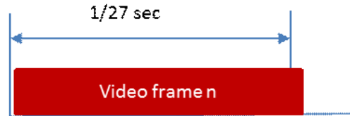
Figure 29 Clock Too Slow - Failure to Read an Entire Frame Within the Frame Period
